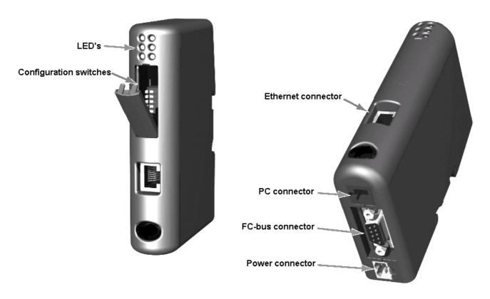
**Configuration switches:** Used for setting IP address.
