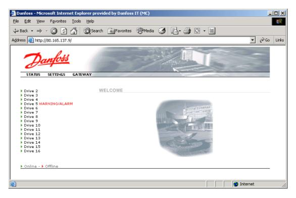
On the main status page it is possible to see all drives connected to the Ethernet Master. By clicking on a specific drive a sub-menu opens, allowing the user to select: **Operating Data**, **Parameter Data** and **Alarms/Warnings**.
